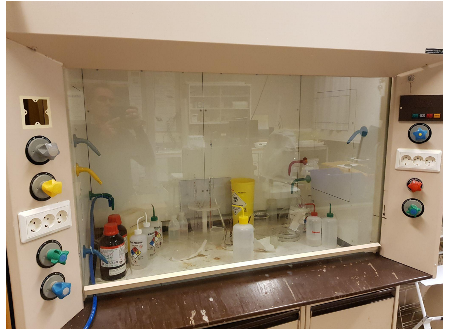
Fume hood for photolithography development
