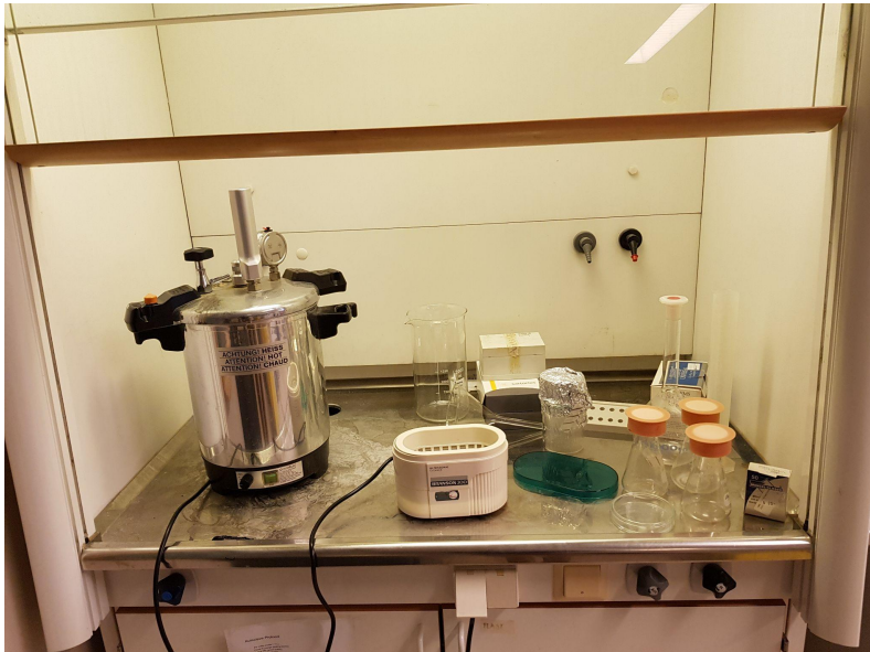
Fume hood with autoclave and ultrasound cleaner
