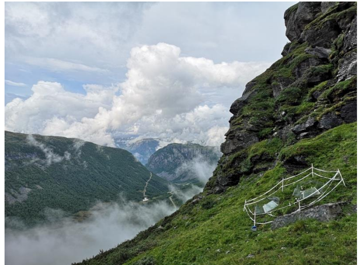
Figure 10. Open-top chambers warm up some of the alpine vegetation plots in Låvisdalen, Vestland (SeedClim site), 2019, photo credit: Eva Lieungh.
