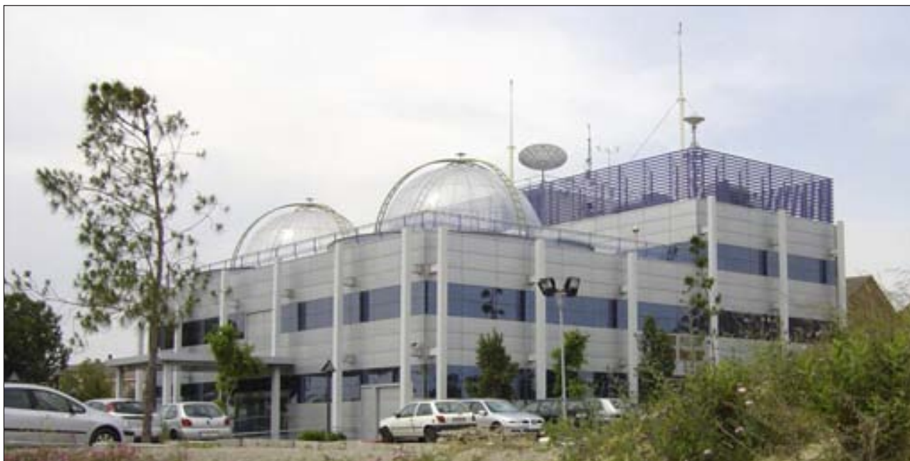
The European Photochemical Reactor, EUPHORE, in Valencia (Spain). There are two Teflon domes in which photochemical experiments can be carried out under natural conditions. Each dome is equipped with state-of-the-art analytical instrumentation for on-line and in situ monitoring of chemical compounds.
