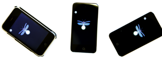
Figure 3.1: Decentralized oscillators modelled as fireflies achieving harmonic synchrony on iOS devices, after starting flashing unsynchronously. Image: K. Nymoen et al. [23].
