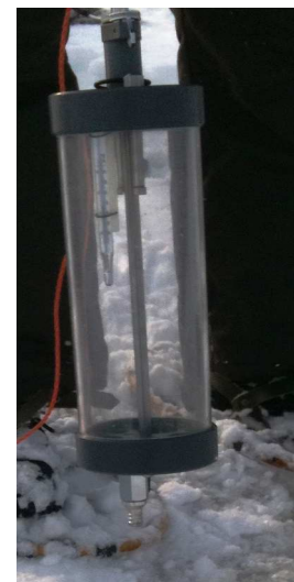
Figure 14. Water sampler device used for Lake Vansjø sampling.
