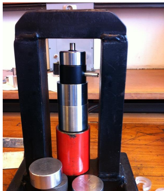
Figure 3: The die mounted on the press platform, and on the table are the rest of the metal cylinders available.
