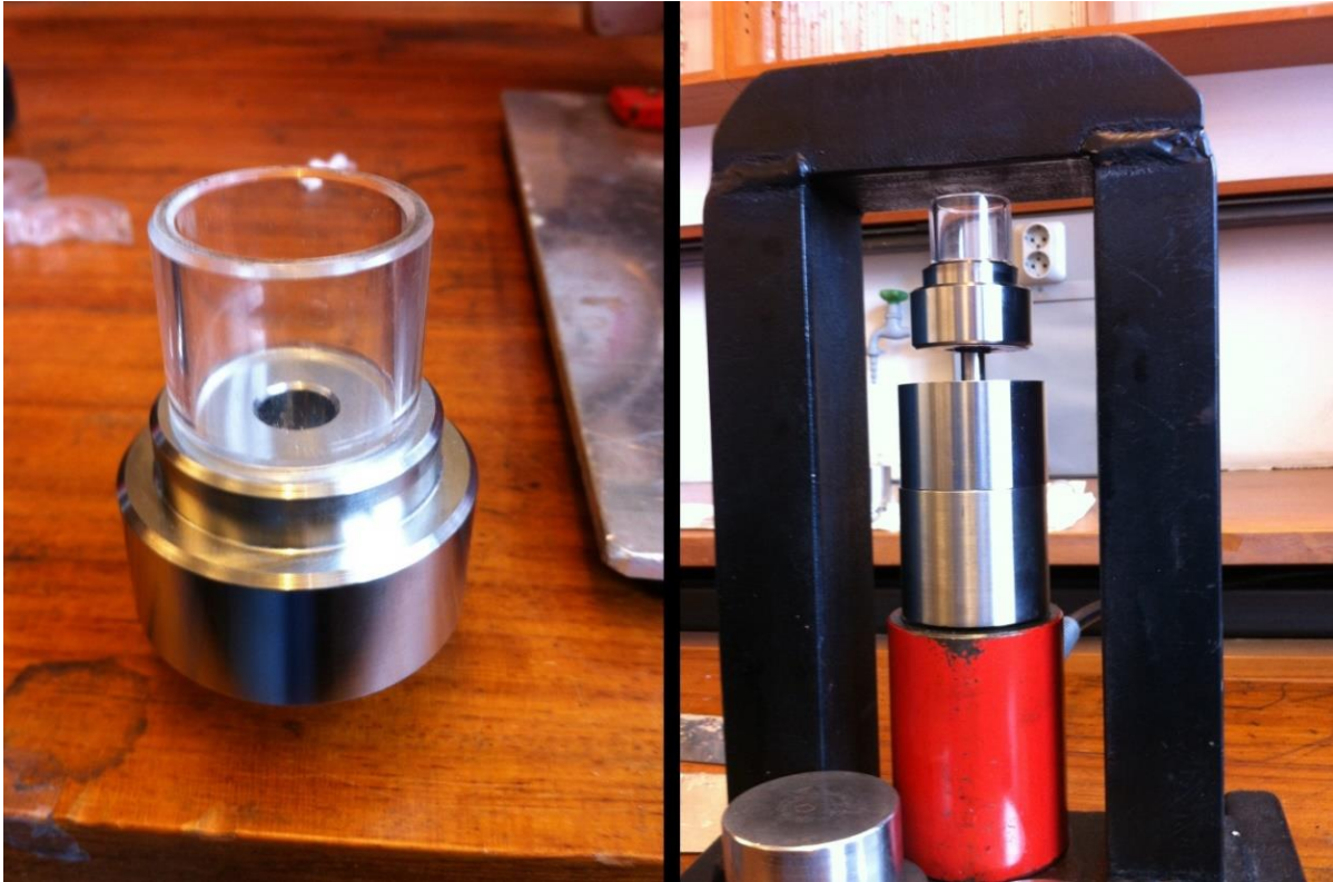
Figure 4: Pictures of how the removal of the pressed pellet should be performed.
