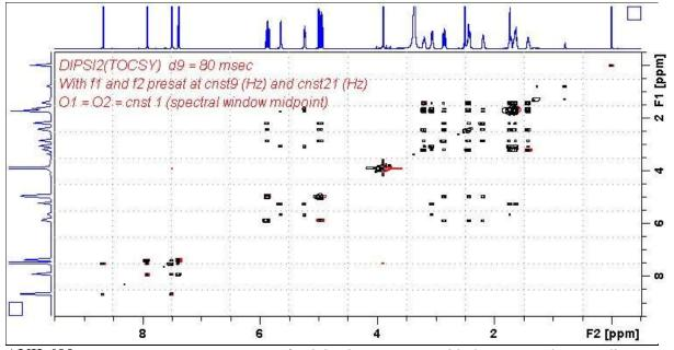
AVII-600 **Dipsi2bfprf1bfprf2** spectrum of quinine in  $D_6$ -DMSO with the HOD and DMSO lines at 3.38 ppm and 2.5 ppm suppressed. The spectrum is centered at 4.5 ppm (O1 = O2 = CNST 1 = 2700.59 Hz).
