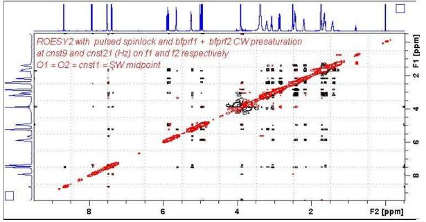
AVII-600 Roesy2bfprf1bfprf2 spectrum of quinine in  $D_6$ -DMSO with the HOD and DMSO lines at 3.38 ppm and 2.5 ppm suppressed. The spectrum is centered at 4.5 ppm (O1 = O2 = CNST 1 = 2700.59 Hz).
