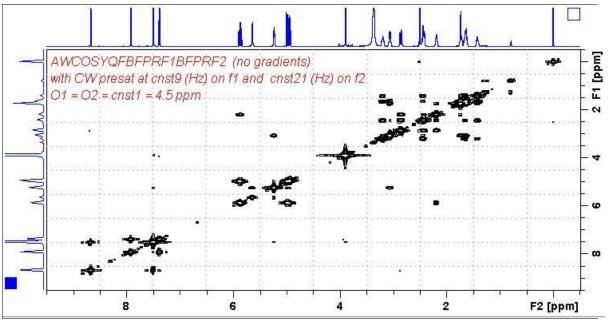
AVII-600 **Cosyqfbfprf1bfprf2** spectrum of quinine in  $D_6$ -DMSO with the HOD and DMSO lines at 3.38 ppm and 2.5 ppm suppressed. The spectrum is centered at 4.5 ppm (O1 = O2 = CNST1 = 2700.59 Hz).
