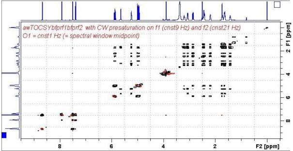
AVII-600 **Tocsybfprf1bfprf2** spectrum of quinine in  $D_6$ -DMSO with the HOD and DMSO lines at 3.38 ppm and 2.5 ppm suppressed. The spectrum is centered at 4.5 ppm (O1 = O2 = CNST1 = 2700.59 Hz).
