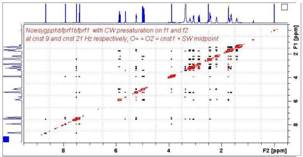
AVII-600 **Noesybfprf1bfprf2** spectrum of quinine in  $D_6$ -DMSO with the HOD and DMSO lines at 3.38 ppm and 2.5 ppm suppressed. The spectrum is centered at 4.5 ppm (O1 = O2 = CNST 1 = 2700.59 Hz).
