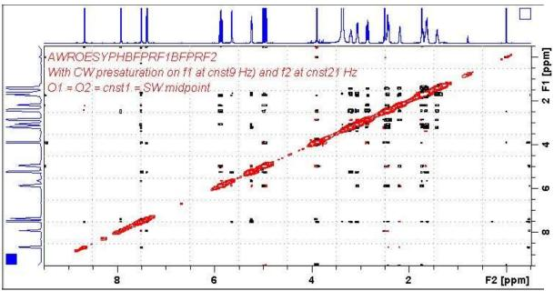
AVII-600 Roesybfprf1bfprf2 spectrum of quinine in D<sub>6</sub>-DMSO with the HOD and DMSO lines at 3.38 ppm and 2.5 ppm suppressed. The spectrum is centered at 4.5 ppm (O1 = O2 = CNST1 = 2700.59 Hz).
