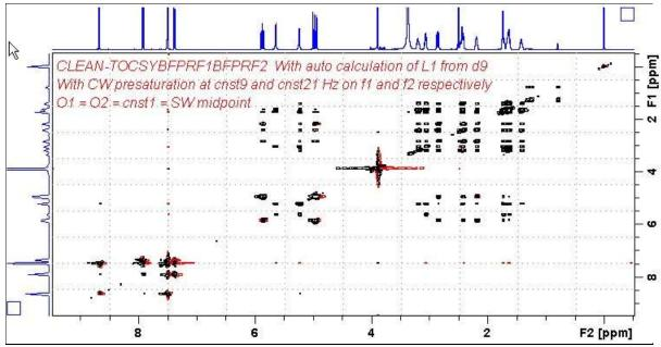
AVII-600 Clean-tocsybfprf1bfprf2 spectrum of quinine in  $D_6$ -DMSO with the HOD and DMSO lines at 3.38 ppm and 2.5 ppm suppressed. The spectrum is centered at 4.5 ppm (O1 = O2 = CNST 1 = 2700.59 Hz).
