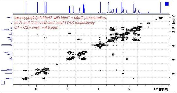
AVII-600 **Cosybfprf1bfprf2** spectrum of quinine in  $D_6$ -DMSO with the HOD and DMSO lines at 3.38 ppm and 2.5 ppm suppressed. The spectrum is centered at 4.5 ppm (O1 = O2 = CNST 1 = 2700.59 Hz).
