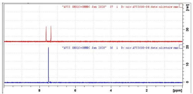
**AVII-600 SELHSQC** (*lower*) and **SELHSQCND** (*upper*) spectra determined for quinine in D<sub>6</sub>-DMSO with selective excitation of the  $^{13}$ C signal at 102.4 ppm (O2 = 15534 Hz).
