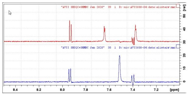
Expansion of the 7.0-8.5 ppm region of the **AVII-600 SELHSQC-DIPSI2** (*lower*) and **SELHSQCND-DIPSI2** (*upper*) spectra determined for quinine in D<sub>6</sub>-DMSO with selective excitation of the  $^{13}$ C signal at 102.9 ppm (O2 = 15534 Hz).
