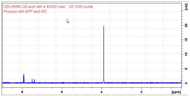
AVII-600 **SELHMBCQ5** spectrum determined for the signal which occurs at 156.4 ppm.
