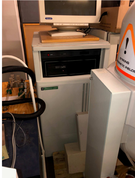
Two Varian Gemini 200 MHz Electronics consoles. One with temperature controller. One upgraded to year 2000 electronics.
