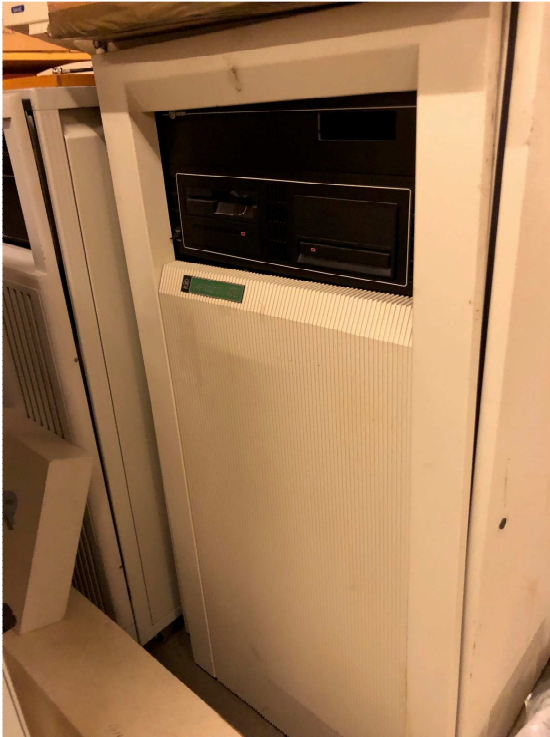
Two Varian Gemini 200 MHz Electronics consoles. One with temperature controller. One upgraded to year 2000 electronics.
