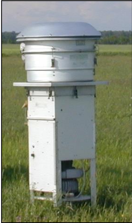
Sierra Andersen Sampler 1000 l/min -1
