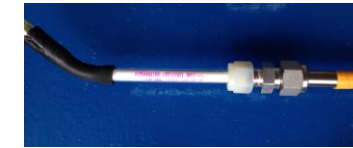
XAD-2 and charcoal sorbent tubes
