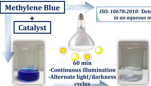
ISO: 10678:2010: 'Determination of photocatalytic activity of surfaces in an aqueous medium by degradation of methylene blue'
