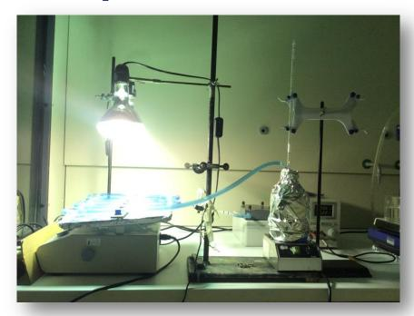
This first prototype will be used to treat turbid wastewater (e.g. olive vegetation waters)
