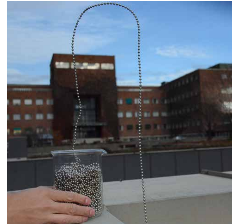
A remarkable self-sustained arch is formed when a long chain of metallic beads is dropped from a container (placed approximately 5m above the ground in this experiment). In the background we see the Physics Department at the University of Oslo.
