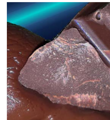
Fig. 2: A material (chocolate) deformed in a brittle way at low room temperature (top right), or in a ductile way (in the bulk) at higher room temperature (left).
