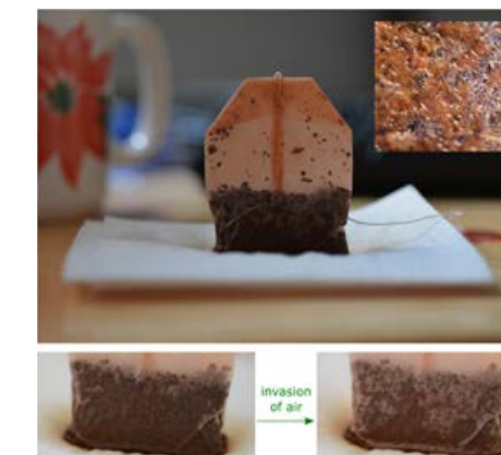
Fig. 1: The tea bag experiment. As the wet tea bag dries, pockets of air suddenly invade the voids (pores) between the leaves, in a typical example of the intermittent burst activity observed in drainage experiments. The inset on the top right shows a macro image of the porous matrix.
