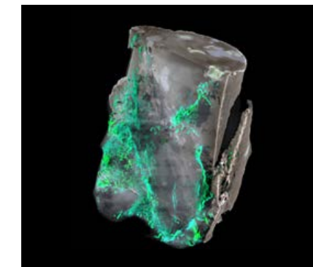
Fig. 1 (above): X-ray microtomography image of fractures in a 5 mm diameter crystalline rock sample (beamline ID19, ESRF). The fracture network (in green) is used as an input for flow simulations. Courtesy of B. Cordonnier.
