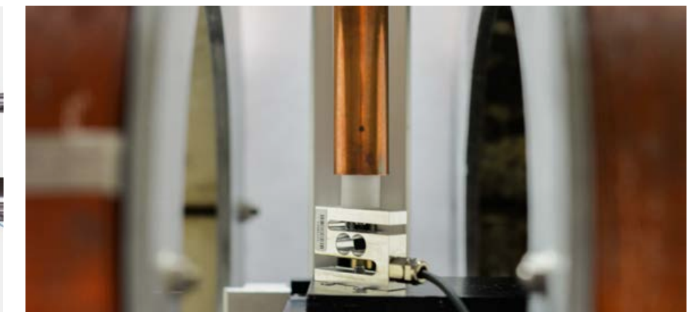
Fig. 2: Measurement of the Janssen coefficient under an external magnetic field generated by two coils in a horizontal Helmholtz configuration. A ferromagnetic grains assembly is filled inside a tube and moved down by a piston mounted on a mass sensor.
