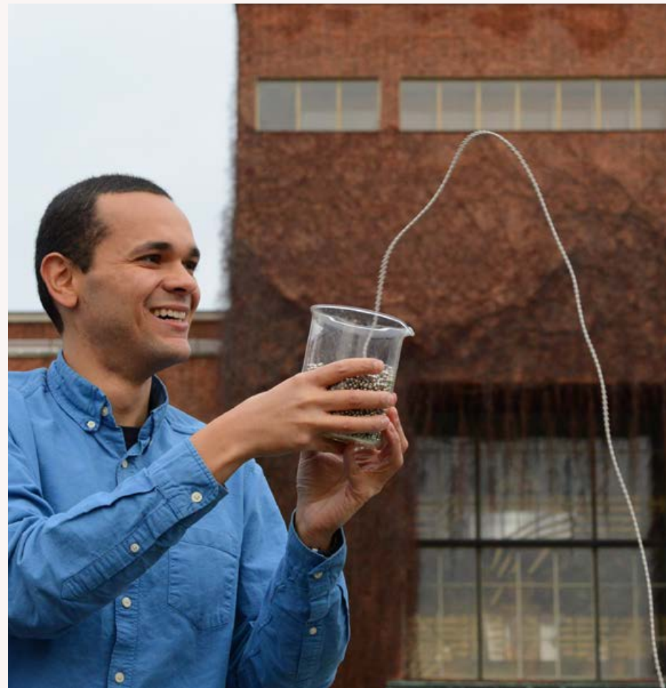
Fig. 1: A remarkable self-sustained arch is formed when a long chain of metallic beads is dropped from a container. The chain reaches a statistical steady state but fluctuations along its length are always present, as seen in the image. In the background we see the Physics Department at the University of Oslo. Picture credit: Hilde Lynnebakken.
