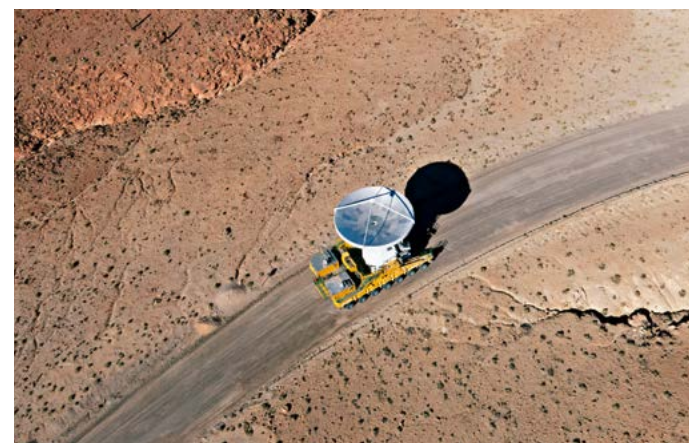
The ALMA 12m antennas can be relocated in different array configurations with different sizes and resulting angular resolution. On this picture, a 12m antenna is transported to its new location.
