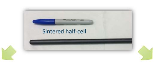
Line 3: based on one end-closed porous BZY extruded tube, on which segments of cathode, electrolyte, and interconnect are sequentially applied and co-sintered.
