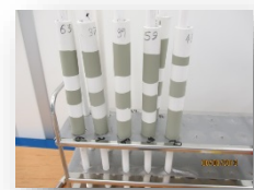
Semi-automatic dip-coater for 1 m long sample (batch of 8 samples)
