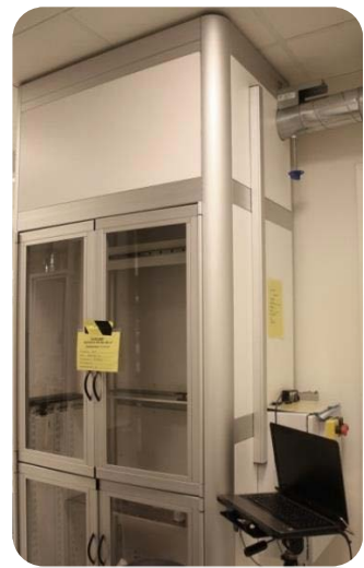
Semi-automatic dip-coater for 1 m long sample (batch of 8 samples)
