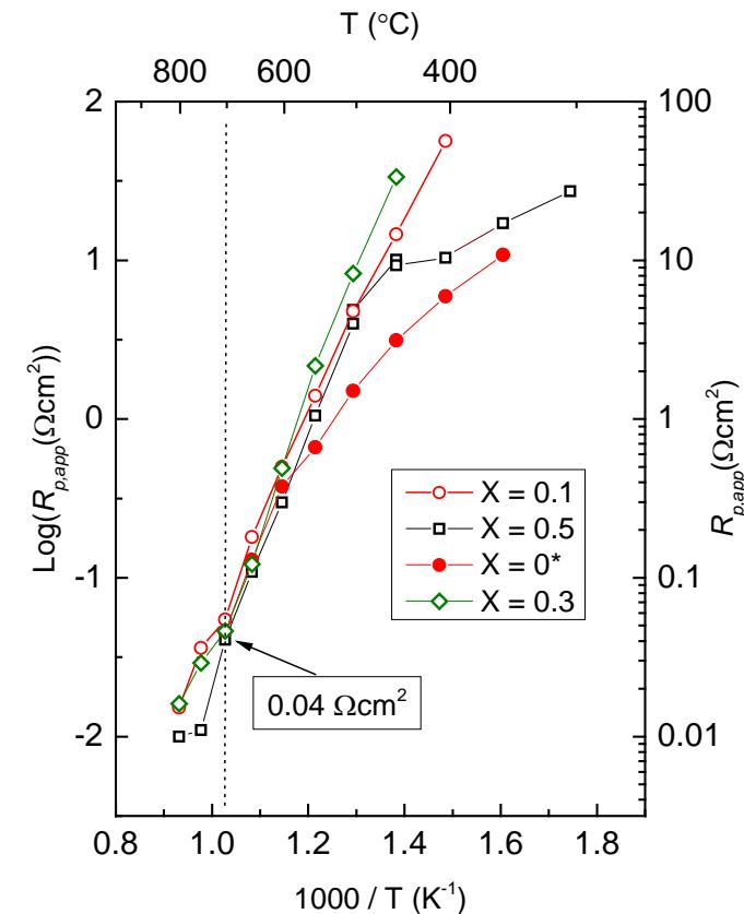
$\text{Ba}_{1-x}\text{Gd}_{0.8}\text{La}_{0.2+x}\text{Co}_2\text{O}_{6-\delta}$  displays best PCE steam electrode performance
