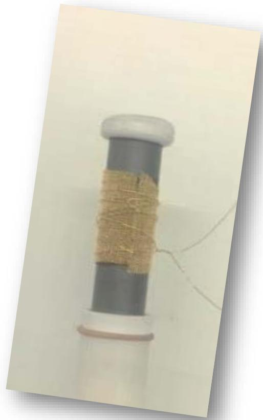
Post-characterization: poor electrode adhesion
