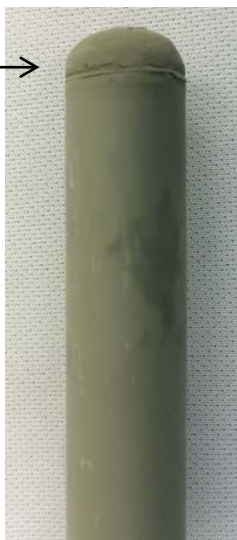
Tubes after extrusion and roll-drying in air for 24h
