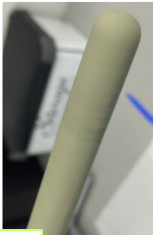
Dried tubes after polishing with wet clean room tissue
